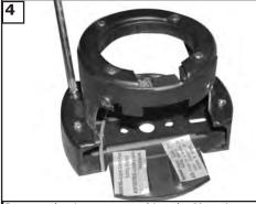
Remove the 4 screws attaching the Mounting neck to the mounting plate. Retain the 4 screws for re-assembly.
